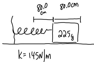
a) The maximum velocity occurs when the kinetic energy is a maximum and the potential energy is a minimum (i.e. at the equilibrium position)
